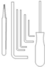
Tool kit with all necessary allen keys, M3 driver, and a pair of tweezers (useful when preparing to print).
