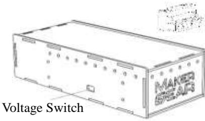
Power Supply—Please read instructions to ensure that your **voltage is correctly set before** powering on. Connects to printer with 6 Position Power Supply Connector.
