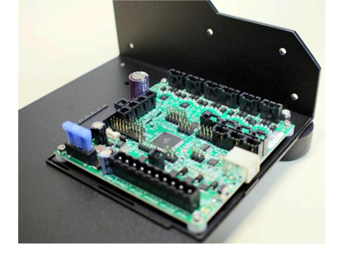
Locate the extended M4 bolt securing the front-right rubber foot to the bottom of the frame; the hole in the front right corner of the RAMBo case BOTTOM piece fits over this bolt. Install and secure the M4 Nylock locknut to secure the BOTTOM in place.
