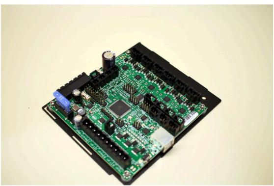
Position the (4) 3/8"x1/8" Nylon spacers over the four tapped holes in the RAMBo case BOTTOM piece, then place the RAMBo on top. Install and secure the (4) #4-40 bolts through the corner mounting holes of the RAMBo, with the spacers in between; do not over-tighten.
