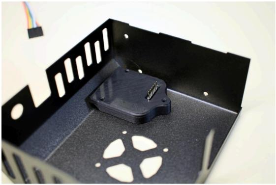
Insert and tighten securely the (3) M3x12mm bolts; as these thread into the printed SD reader holder, do not over-tighten.
