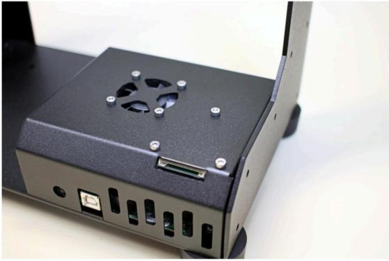
The RAMBo case TOP piece fits over the electronics, flush against the inside right edge of the frame.
