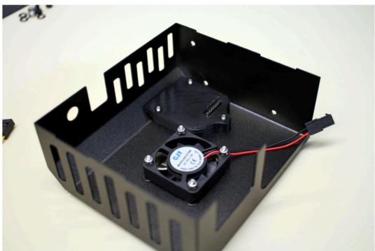
Flip the TOP over; place the (4) M4 black oxide washers and (4) Silver 3/8 washers over the (3) M3x18mm bolts, then position the fan with the wires extending towards the SD reader. Install and tighten the (4) M3 Nylock locknuts.
