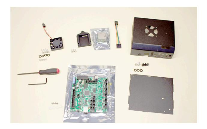
This shows the components of the metal RAMBo case, and those necessary to properly install it:
