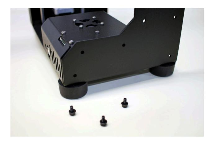
(3) M4x8mm black oxide bolts secure the TOP piece to the frame.
