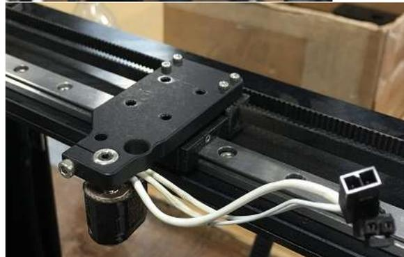
Place washers on two m3 x 10 bolts and secure the black metal motor mount plate to the carriage through the rear two holes using a 2.5 mm wrench.
