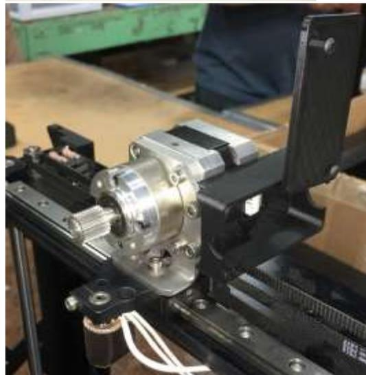
Re-install the filament drive with the m3 x 12 bolts that were securing it previously through the holes to the top left and bottom right of the drive gear using a 2.5 mm wrench.
