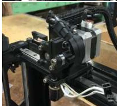
Remove the filament drive from the extruder motor using a 2.5 mm wrench to loosen the screws to the top left and bottom right of the drive gear.
