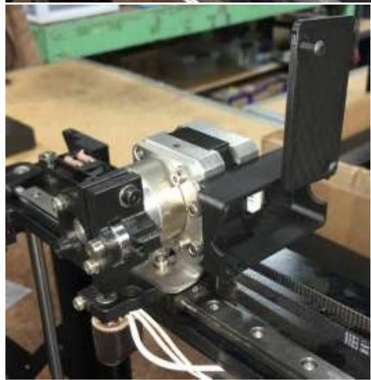
Re-install the fan assembly with the m3 x 45 through the bottom left corner of the 40 mm fan (smaller fan) using a 2.5 mm wrench.
