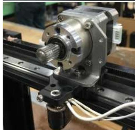
Attach the junction box cover to the junction box through the top right corner with 1 black m3 x 10 button head using a 1.5 mm wrench. Rotate the cover 90° so that it is out of the way for subsequent steps.
