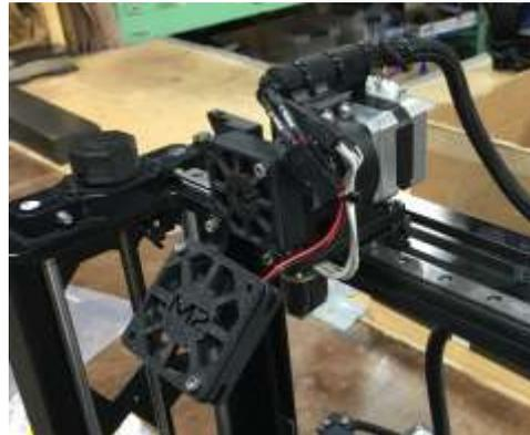
Snip and remove the three cable ties securing the plastic extruder motor mount cover and the one cable tie securing the hot end and fan wires (on the side of the filament drive).
