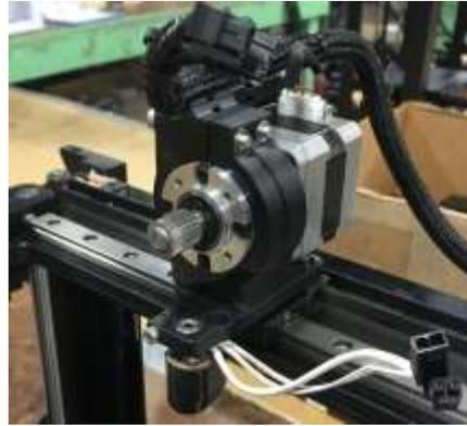
Disconnect the harness from the motor.
