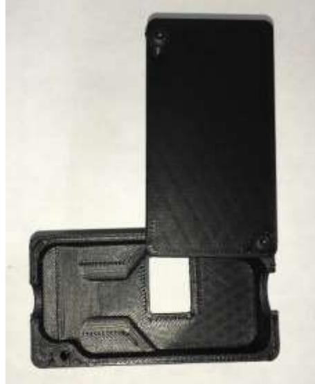
Place the junction box on the side of the extruder and secure to the metal motor mount with two m4 x 16 bolts using a 3 mm wrench.
