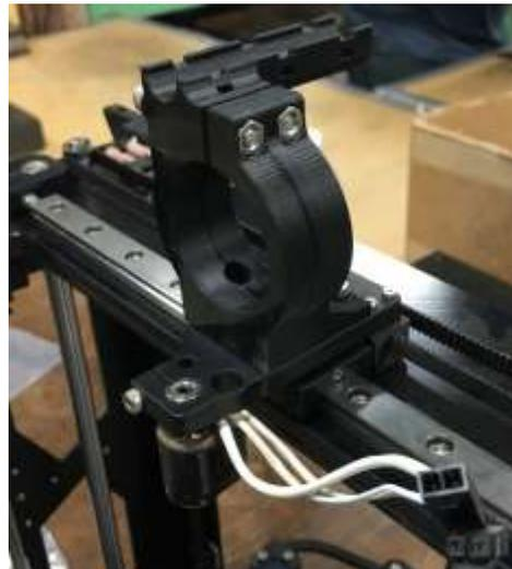
Remove the extruder motor mount by unscrewing the four m3 bolts using a 2.5 mm wrench.
