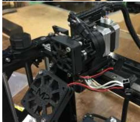
Remove the fan assembly from the filament drive using a 2.5 mm wrench to loosen the M3 bolt in the bottom left corner of the 40 mm fan (the smaller fan).
