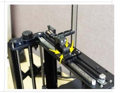
Once the printed Extruder Motor Mount is removed, use two M3x10mm bolts, with washers, to secure the acrylic Extruder Motor Plate to the X Carriage (IN YELLOW).
