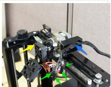
Install the Wire Shroud side panel (making sure the wires are in the slots, at front and rear - IN YELLOW) by using your 2mm Allen wrench to tighten the two M3x10 black oxide button head bolts (IN BLUE).
