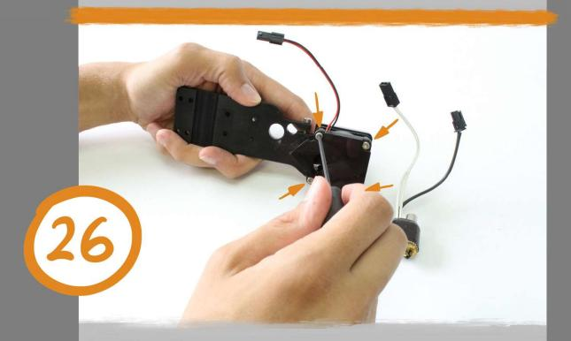
Loosen the four (4) M3x25mm screws from the hotend fan assembly.
