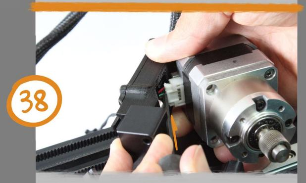
To connect the motor, line it up with its cable, the connector is polarized and will only go in if the 'U' shape is facing forward. After they are lined up, you can use one of your drivers to push the connector until is fully seated in the motor as pictured in the next step.
