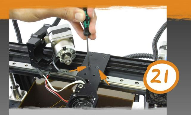
Use a 2 mm hex driver to remove the two (2) M3x10 flat head screws from the hotend mounting plate.
