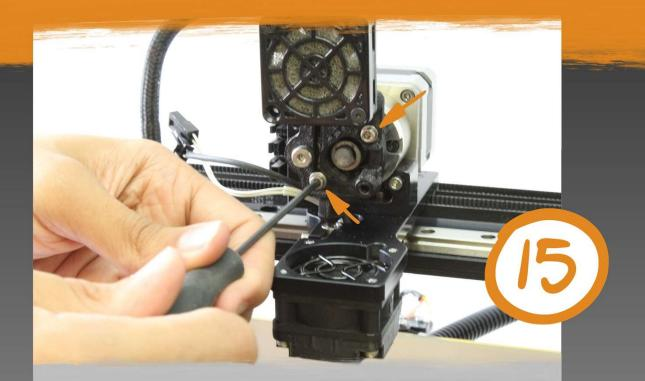
Use a 2.5 mm hex driver to remove the two (2) M3x25mm screws from the filament drive. These screws have M3 washers on them so make sure they stay together.
