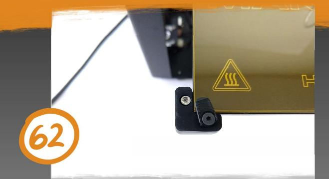
The bed clips should be tight enough that the bed doesn't move side to side freely. They should also be angled toward the corner of the glass as shown above.
