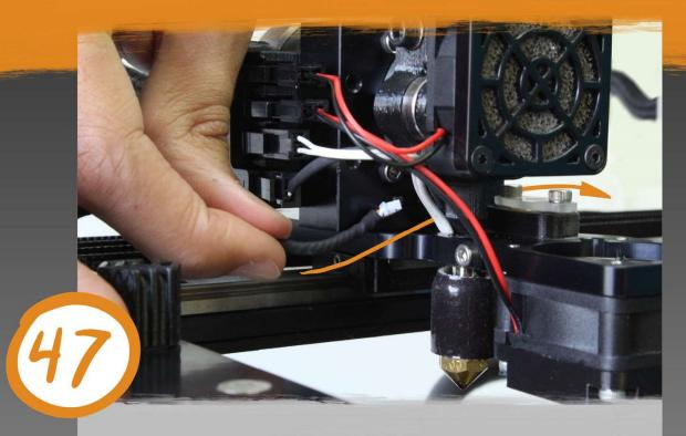
Locate your BL Touch harness and pass it under the left side of the filament drive as shown.
