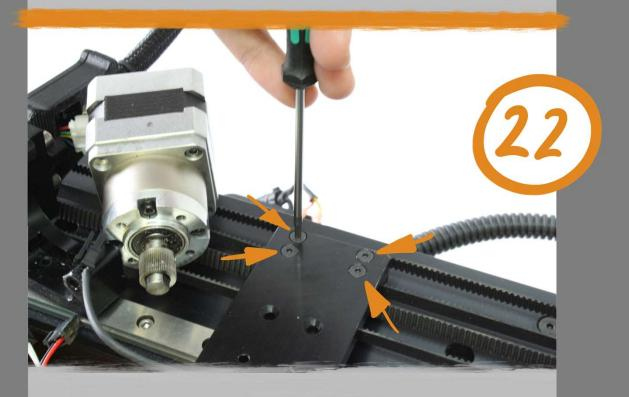
Use a 2 mm hex driver to remove the four (4) M3x16 flat head screws from the hotend mounting plate.
