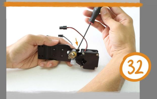
Slide the hotend into the clamp and tighten it with a 2.5 mm hex driver so that the top of the hotend is flush with the top of the hotend mounting plate.
