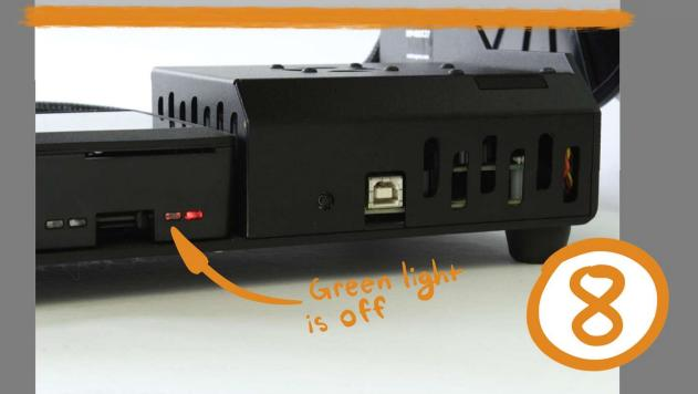
The raspberry pi's green light will turn off when it is properly shut down.
