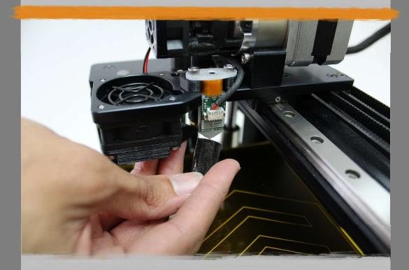
Slip the sleeve over the bottom of the sensor.
