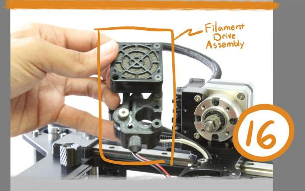
Now the filament drive assembly is free and can be set aside for later use.
