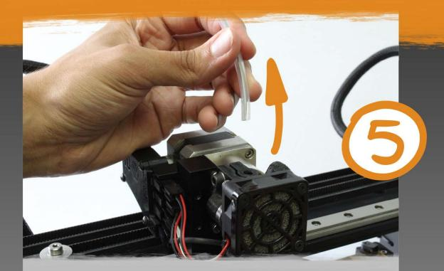
Remove the filament and filament guide tube from 'T0'.
