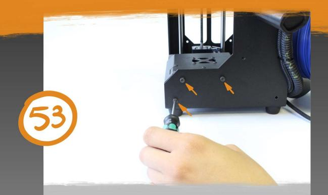
Use a 3 mm hex driver to loosen the three (3) M4x8 screws from the right side of the printer.
