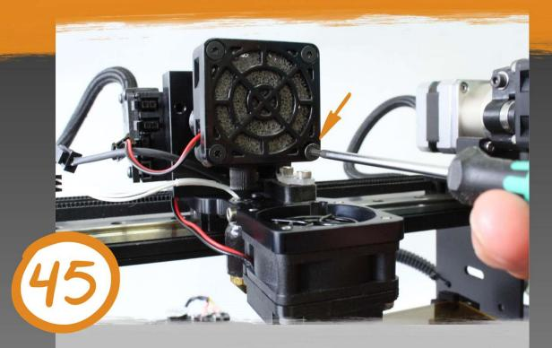
Rotate the filament driver fan down and fasten it using a 2 mm hex driver and the M3x45mm flat head screw from step 13.
