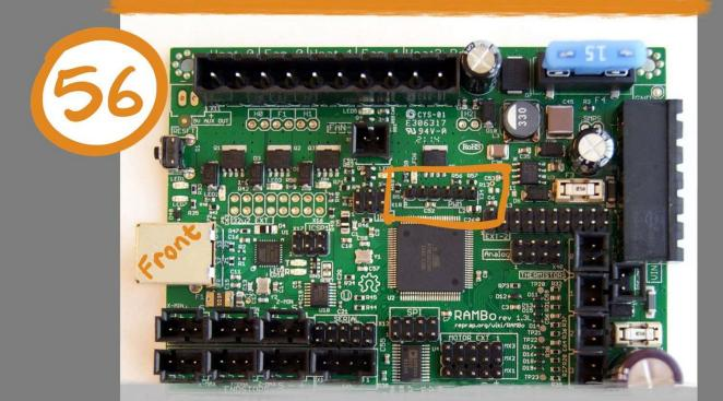
Plug the 6-pin cable housing into the highlighted row of 6-pins. The next diagram will show you the correct orientation.
