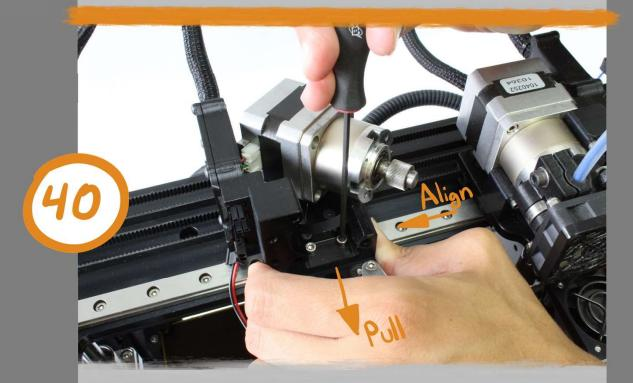
Pull the motor mount forward and line up its right edge with the edge of the hotend mounting plate. Just using a finger to feel for when they are coplanar is enough. While holding it in this position, tighten down the two screws completely.
