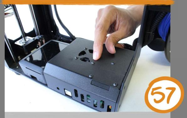
Replace the RAMBo case top. Use your finger to make sure the RAMBo case fan can still move freely. If it doesn't then rearrange the cables inside by just flexing them away from the fan.
