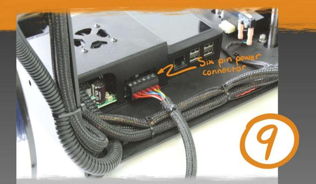
Locate your 6-pin power connector in the back of your printer.
