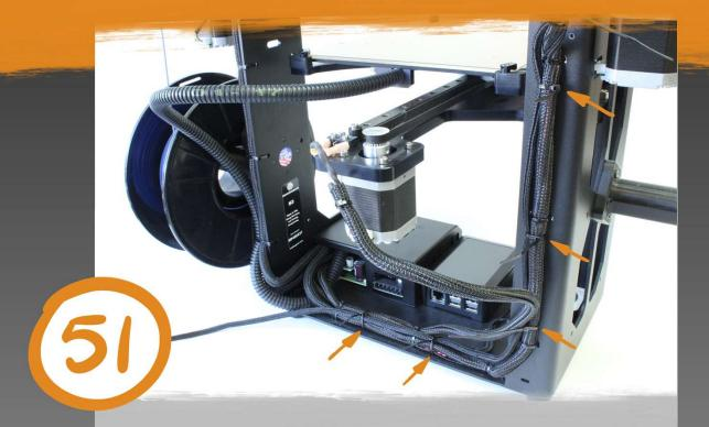
Pass the zip ties between the original harnesses and the frame until the BL Touch harness is secured all the way to the back of the RAMBo case.
