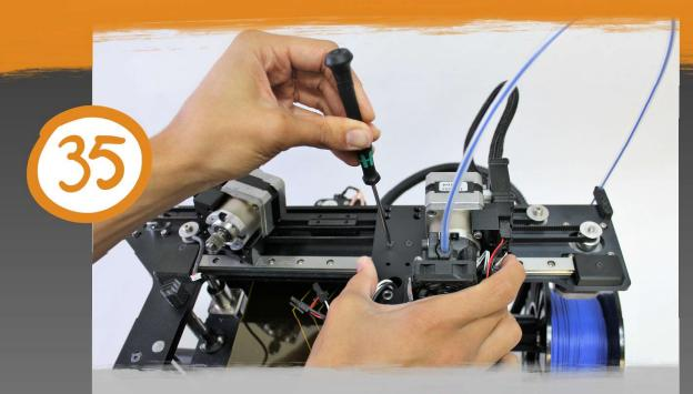
Move T0 and T1 by hand and press them together. While they are being pressed together, tighten the two screws completely. This will ensure that T0 is straight. When tightening multiple screws make sure all of the screws are loosely fastened before fastening all of them completely.
