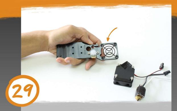
Place the finger guard into the bottom of the new hotend mounting plate. The raised side of the finger guard should be towards the top of the new hotend mounting plate.
