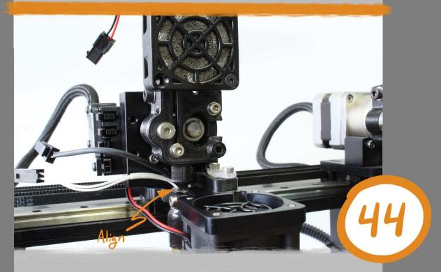
Make sure the exit for the filament drive is visually lined up with the entrance to the hotend.
