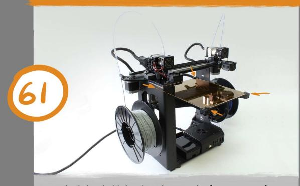
Your bed clips hold the glass down at the four corners of your bed. Remove your old bed clips using a 2 mm hex driver to unscrew the M3x22mm flat head screws. Then install the new ones with the same screws.
