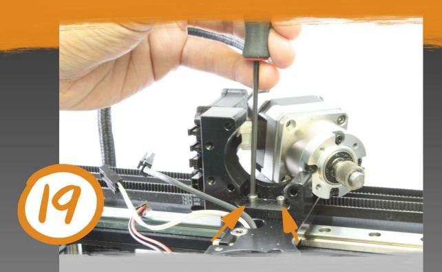
Use a 2.5 mm hex driver to remove the two (2) M3x14mm screws from the motor mount.
