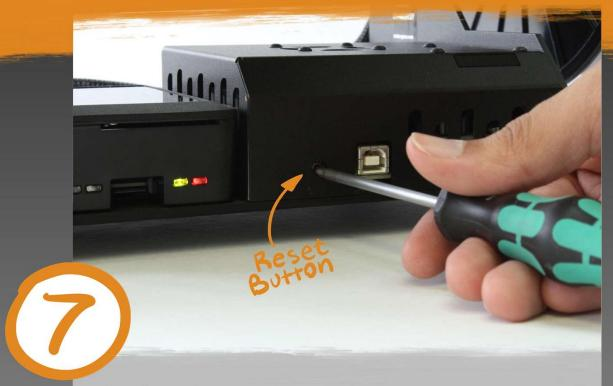
Shut down the printer's raspberry pi through Octoprint or by holding down the reset button for 10 seconds.
