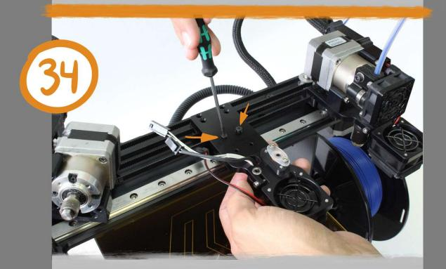
Loosely fasten the hotend mounting plate to the linear carriage with a 2 mm hex driver using the two (2) M3x10mm flat head screws from step 21.
