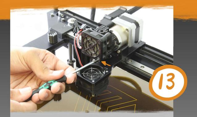
Use a 2 mm hex driver to remove the M3x45mm flat head screw in the bottom-right of the filament drive fan.
