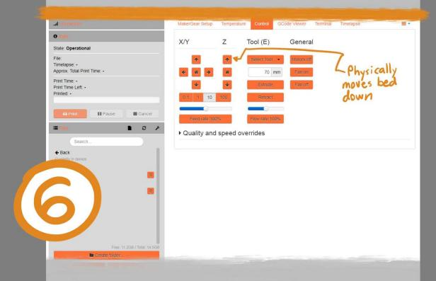
Home the Z-axis with the house shaped button. Move the Z-axis down by around 30 mm (this will give you room to remove the RAMBo case top later).
