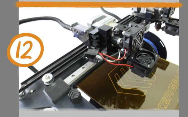
Unplug all of the molex connectors from the extruder. Each one has a lever that needs to be pressed to release the connector.
