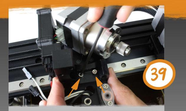
Loosely fasten the motor mount to the hotend mounting plate with a 2.5 mm hex driver using the two (2) M3x14mm screws from step 19.
