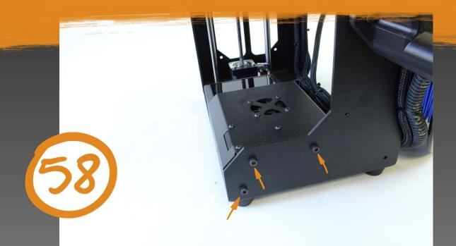
Use a 3 mm hex driver to fasten the RAMBo case top to the frame using the three (3) M4x8 screws from step 53.
