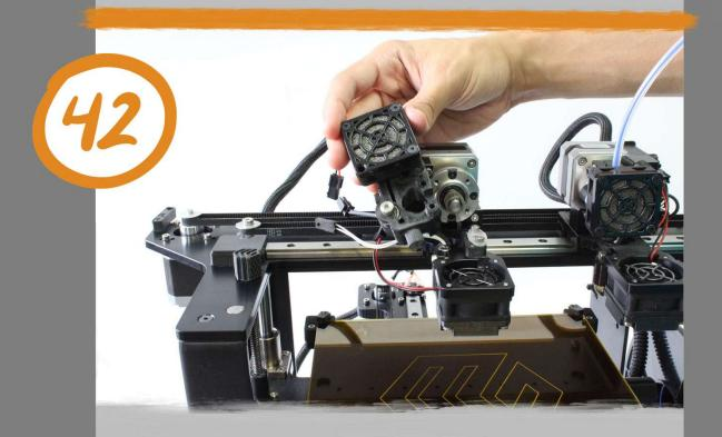
Locate your filament drive assembly from step 16.
