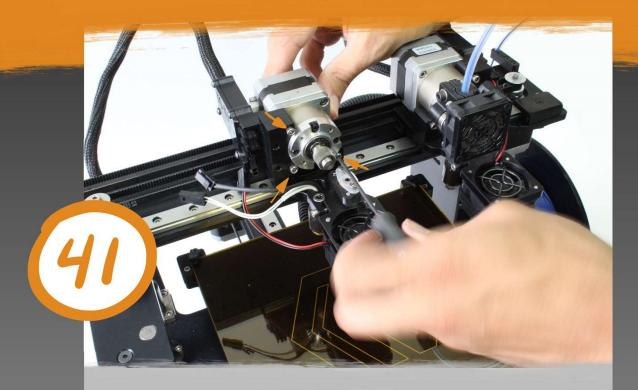
Carefully rotate the motor back into the motor mount and fasten it using a 2.5 mm hex driver with the three (3) M3x25mm screws from step 17.
