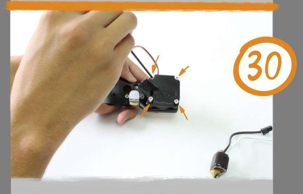
Use a 2.5 mm hex driver to fasten the fan assembly to the hotend mounting plate using the four (4) M3x25mm screws. Make sure the orientation is correct!
