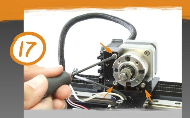
Use a 2.5 mm hex driver to remove the three (3) M3x25mm screws from the motor mount.
