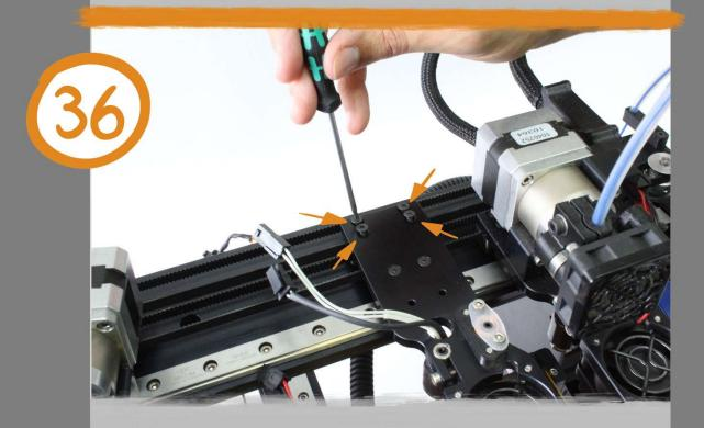
Fasten the hotend mounting plate to the belt clamp with a 2 mm hex driver using the four (4) M3x16mm flat head screws from step 22.
