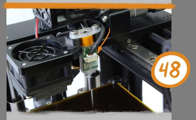
Plug it into the BL Touch. This connection is also polarized so you may need to flip it. The next instructions will show you how to install the insulative sleeve that will protect the sensor from heat.
