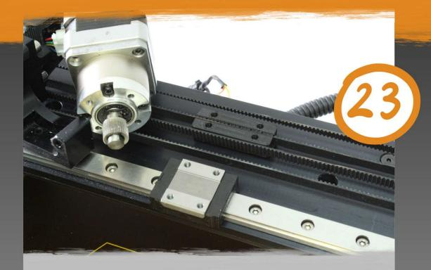
Remove the hotend mounting plate from the printer. Now we are going to move its parts to the upgrade assembly.
