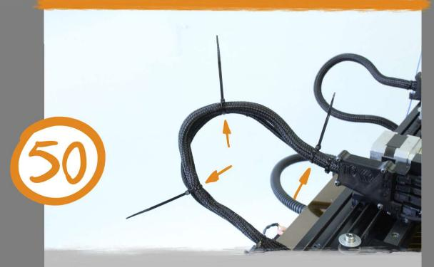
Add zip ties to anchor the BL Touch harness to the original extruder harness. The BL Touch harness should just follow the harnesses arc so zip tie placement isn't exact, but you can use these pictures for reference.
