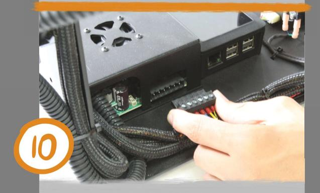
Shut off the printer's 24V power supply and pull out the 6-pin power connector in the back of the printer.
