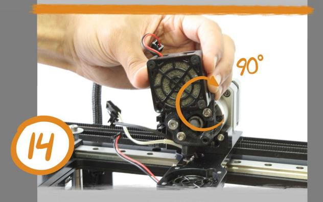
Rotate the filament drive fan clockwise to expose the screw heads beneath.
