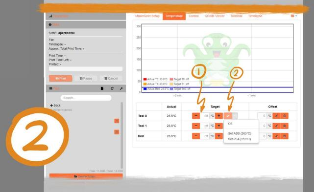
Open Octoprint and heat up your hotend. Set the hotend to the printing temperature of the loaded filament (e.g. ABS: 265 C, PLA: 215 C).
