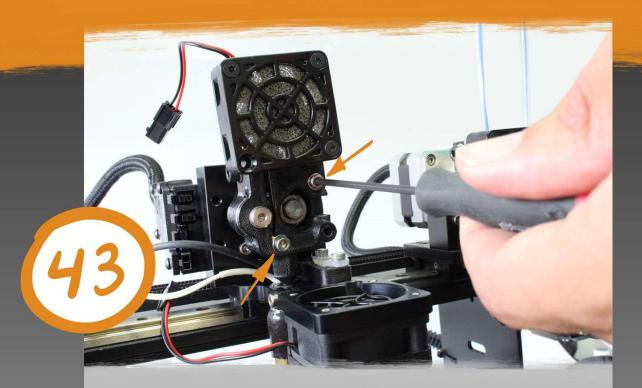
Fasten the filament drive assembly to the motor using a 2.5 mm hex driver and the two (2) M3x25mm screws/washers from step 15.
