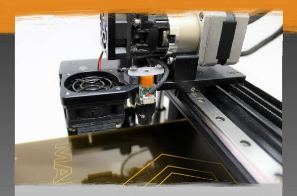
It can be a tight fit so if the sleeve gets stuck on the connector, you can use one of your drivers to widen the opening while pushing up on the sleeve.
