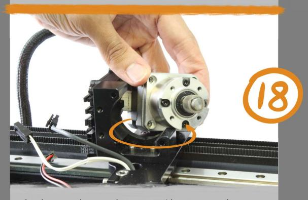
Gently move the extruder motor aside to expose the screws beneath. The motor is connected to a cable; this cable can be left attached to the motor, but if it is detached we have steps for reattachment later.
