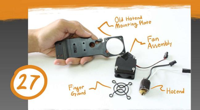
Pull off the fan assembly and finger guard and set it aside.
