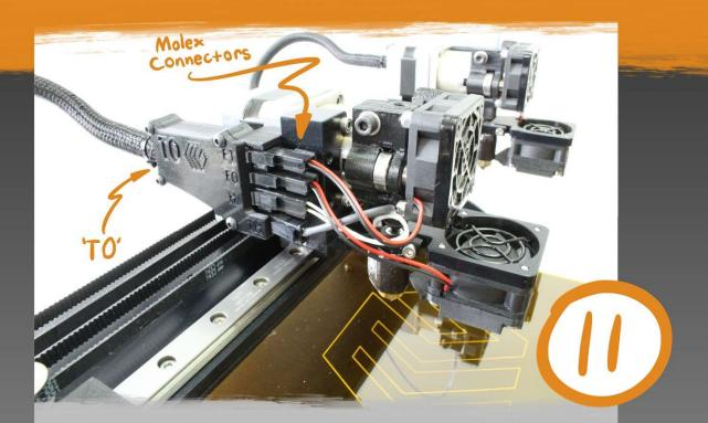
Make sure you are working on the correct extruder! Looking at the front of the printer, we will be modifying the left extruder, it is marked as 'TO'.
