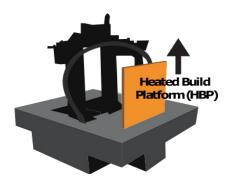
2. Remove foam from above and below the 4-legged "spider" inside the frame. Remove the heated build platform from its slot in the foam and place it on the spider with the glass build plate facing up, as shown on page 5.
