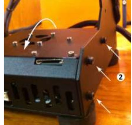
**After making the three connections shown on the next page, replace the electronics cover and lower the bed.**
