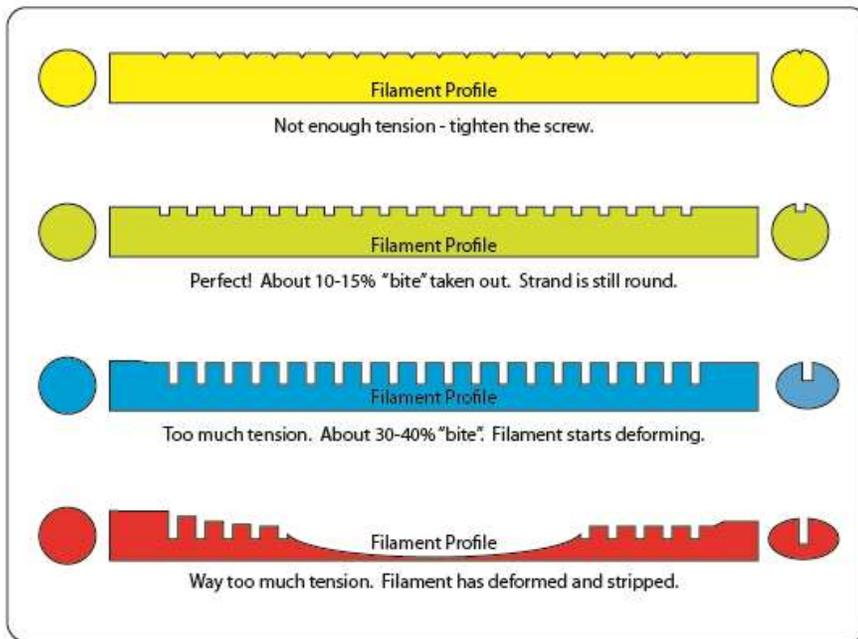
Look at the diagram to determine how to adjust the tension on the screw.
