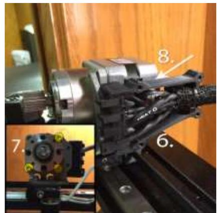
Slightly loosen/straighten the white connector wire to give yourself some working room. It helps to have a fingernail to get underneath the lip on the white connector, or a thin flat screwdriver can help. Gently separate the connector by pulling straight back on the raised lip towards the bracket. (No catch on this one.)
