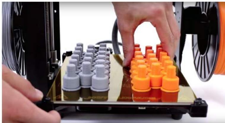
Above: Models printed on rafts and using MakerGear's Mimeo Mode feature to create multiple prints at once.
