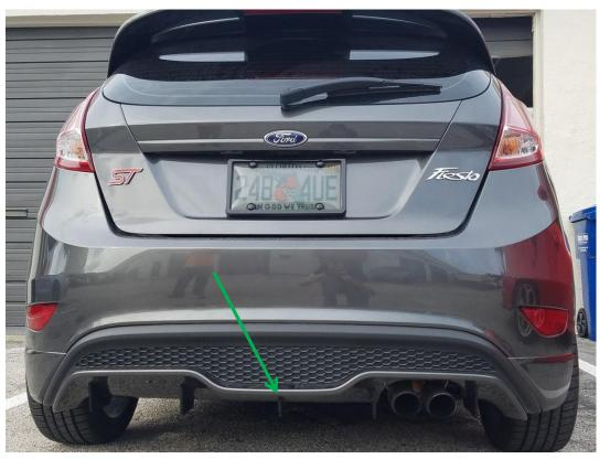
Once you are confident in the placement of the center fin, you can use an erasable marker or piece of painters tape to mark the spot. Remove the adhesive protector from the fin and firmly press the fin onto the bumper, have your friend or marking mechanism ensure it is straight.
