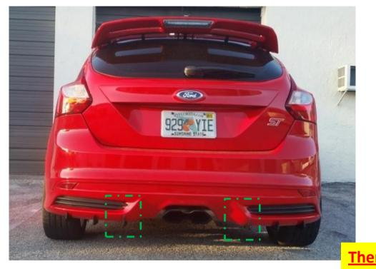
Fin 3 example picture Hook fin behind this spot **There should be NO GAP** between fin and bumper
