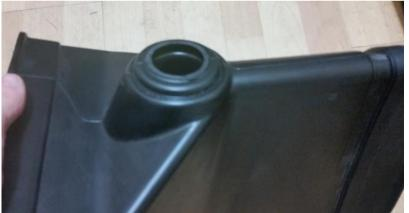
You will need to cut directly ABOVE the small shoulder present at the base of the resonator. Do not cut below the shoulder!
