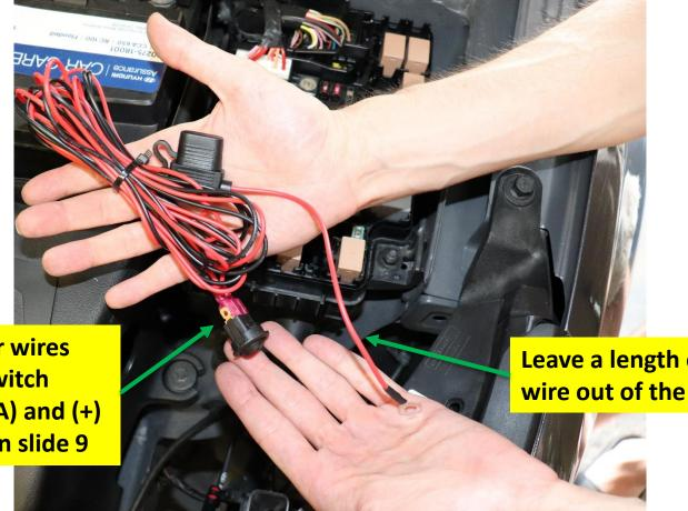
**Both power wires** plug into switch terminals (A) and (+) as shown on slide 9
