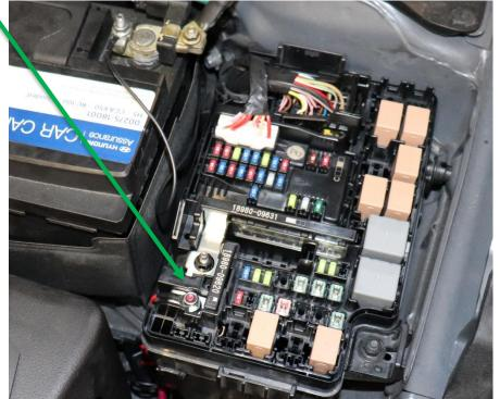
If you would like the switch LED to light up when switch is on, ground the switch using the supplied ground wire.
