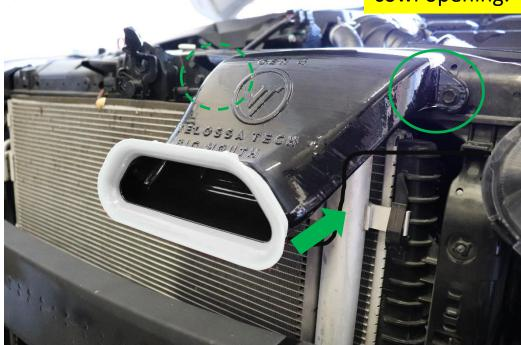
Snake the LED cable in this direction once the BIG MOUTH is installed.
