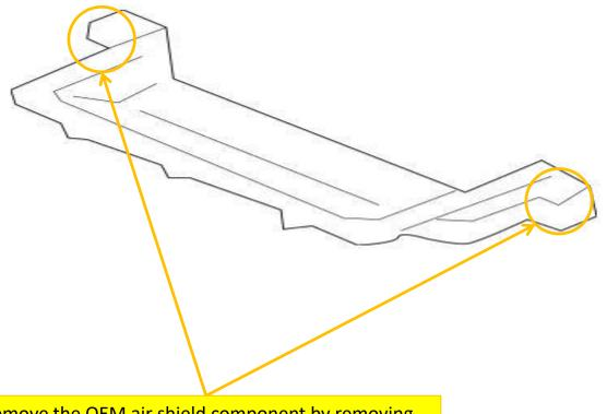
Remove the OEM air shield component by removing the 10mm bolts. This piece will not be reused.
