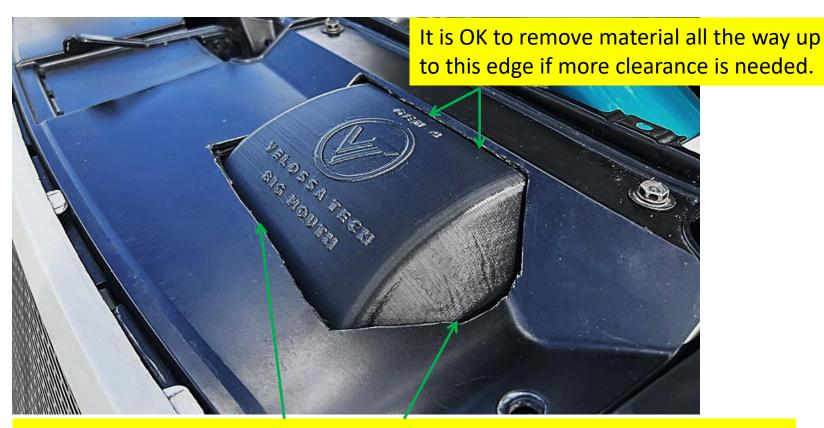
If there is any hard binding, remove more material in any of these places underneath the bumper cover.
