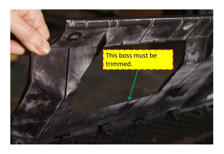
After trimming the cover/shroud, fasten the shroud back underneath the bumper cover. <u>The bumper cover should seat back properly with no serious binding</u>, if not, go back and continue to trim ribs/bosses until the BIG MOUTH and cover are not binding. Trim liberally to ensure no stress on the BIG MOUTH.
