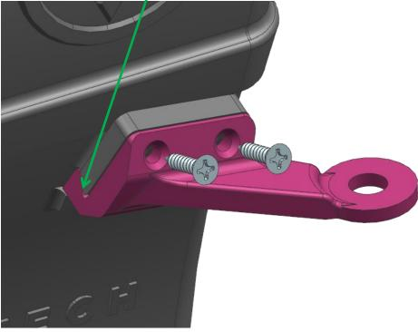
You may slide in bracket 2 from the side to engage the dovetail hook.
