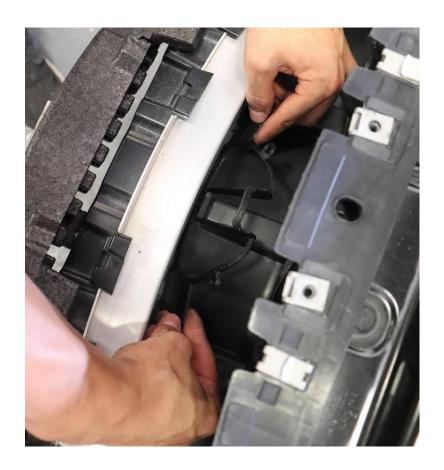
Ensure that the template is seated as shown, and make sure it is pushed as far towards the rear of the car as possible.
