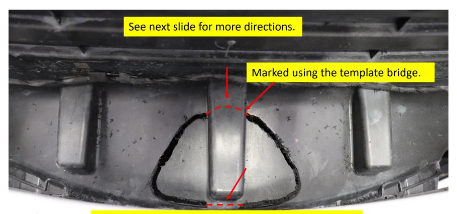
This area will not be able to be marked with the template, just connect both sides with a straight line.
