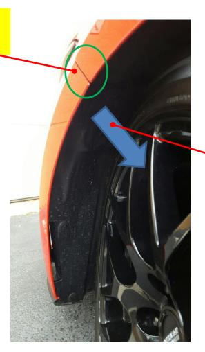
Pull this region of the liner back slightly, it is best to reach in from both the top and bottom to work with the 7mm screw. A swivel and extension helps for this process.
