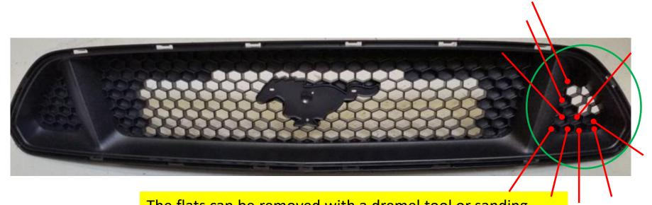
The flats can be removed with a dremel tool or sanding tool, a sharp blade can also be used if done carefully.
