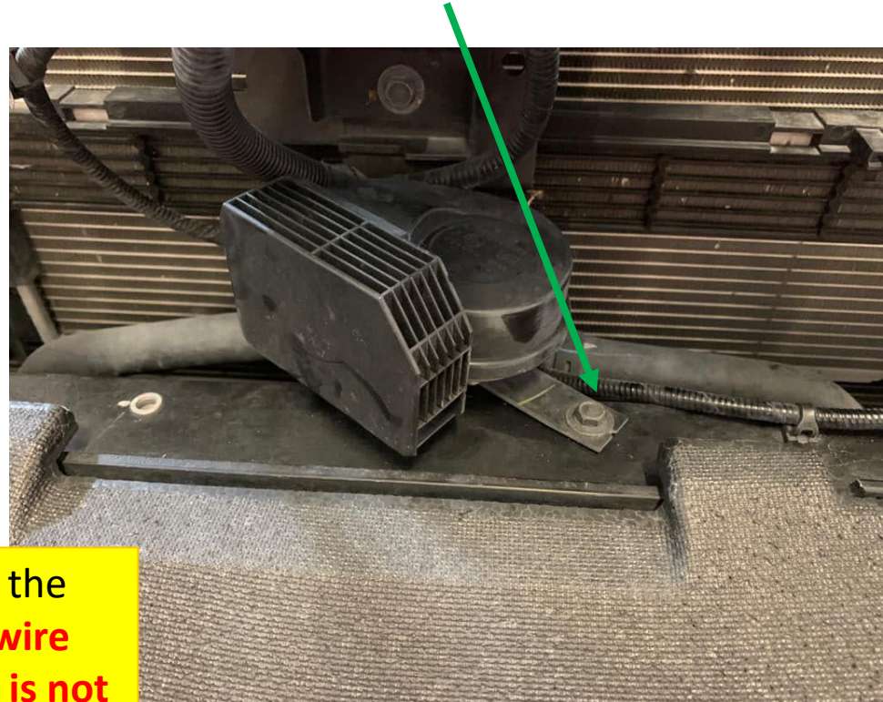
3. Using the same horn bracket, relocate it here and bolt it down using the OEM bolt.
