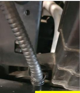
Use pliers to pinch the clip from the rear and pull for release
