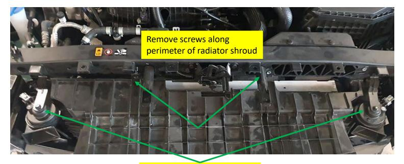
Remove horns in order to make room for radiator shroud removal
