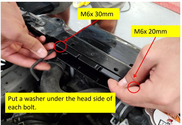
Thread the bolts into the stock threads but **DO NOT TIGHTEN**. It should be loosely attached to allow for incremental movement.
