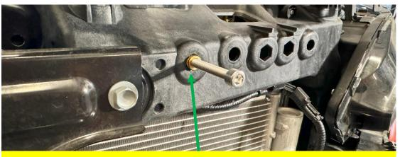
Press fit the provided M6 brass insert into this hole (the insert in this image is NOT flush; press until flush)
