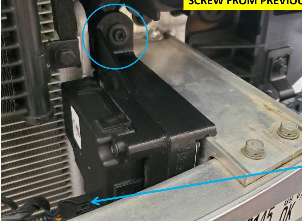
Install the servo casing as shown and **plug the associated connector back in**.
