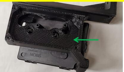
Bring the housing in from the top and slide the 'roof' area under this lever, then go to step 3.
