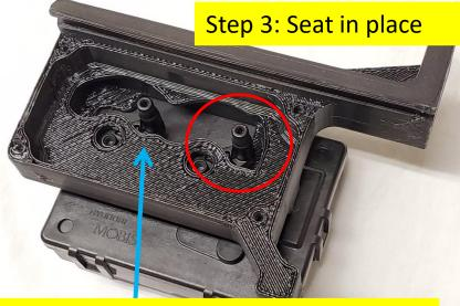
Ensure this lever can move freely, <u>do not</u> <u>try and rotate the right-most lever!!</u>
