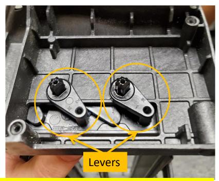
Once the motor is removed, you will see two AGS levers. These levers will need to be removed so they can be re-used in the AGS simulator bracket in the coming slides.
