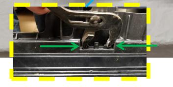
Use channel locks on a wide setting to pinch these clips, keep them pulled back so they don't snap back in place as you move around the shroud.
