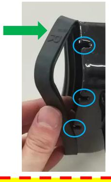
Note that R is RIGHT side (or passenger side) and L is LEFT side (or driver side). They are **NOT** interchangeable and the letters must be pointing up when you reinstall them onto the BIG MOUTH intakes!
