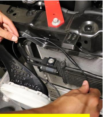
Take notice of the notch within the M8 female connector. The connectors must be properly oriented and should not require very much force to connect. Improper alignment can damage the pins within the male connector.
