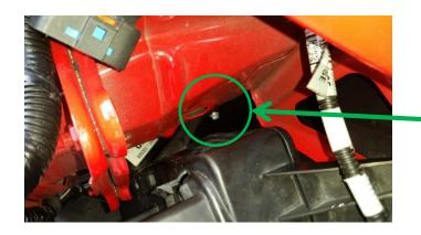
This image is a top down view standing over the driver side fender, the bolt is closest to the engine.
