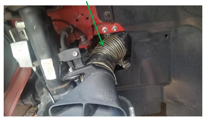
Ensure all hose ends are wrapped completely around the duct adapters, use the supplied stainless steel band clamps to secure.
