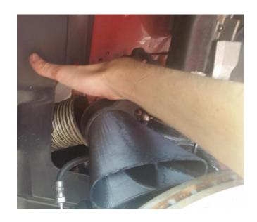
Ensure all hose ends are wrapped completely around the duct adapters, use the supplied stainless steel band clamps to secure.
