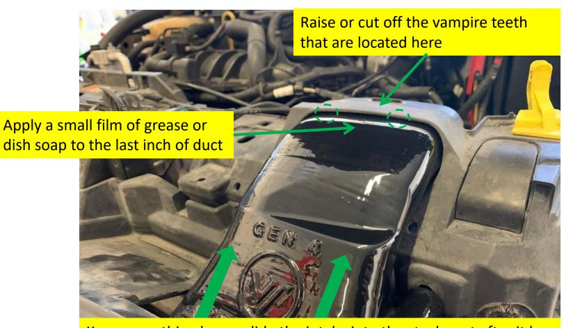
Keep everything loose, slide the intake into the stock port after it has been lubricated. You may apply light pressure to slide it into the stock gasket.
