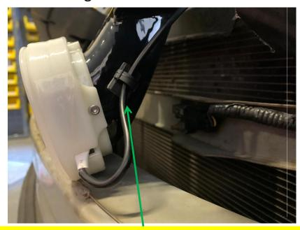
LED power cable must exit the <u>driver side</u> of the flare once installed!
