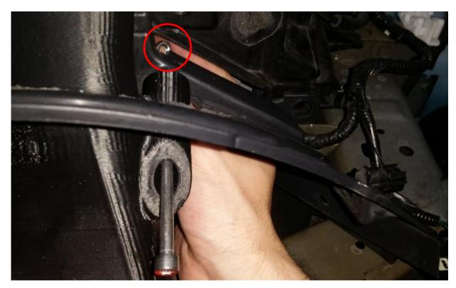
You may want to place the 65mm bolt in the fastening boss to prepare for alignment.
