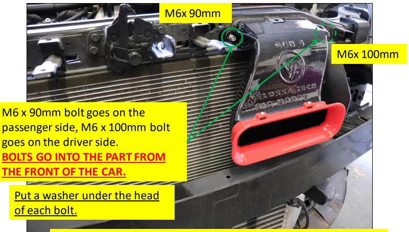
Thread the bolts into the stock threads and tighten snug, **DO NOT OVER TORQUE.**
