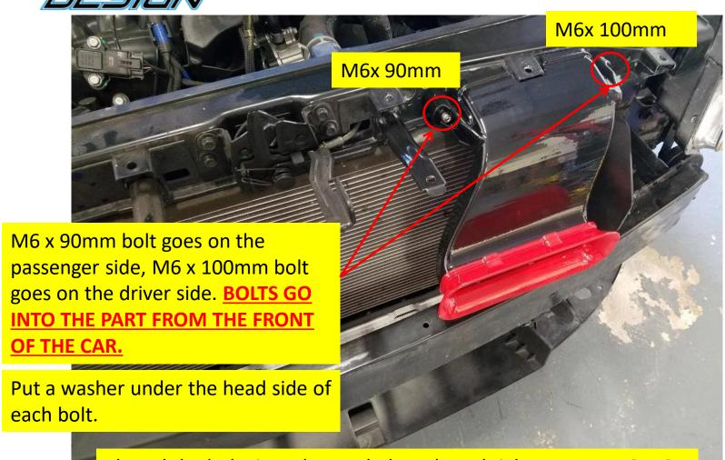
Thread the bolts into the stock threads and tighten snug, **DO NOT OVER TORQUE.**
