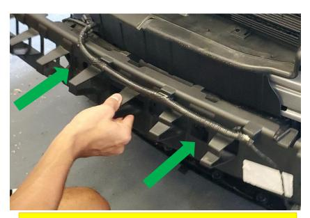
Use the 16" zip ties to fasten the horizontal wire loom to crash bar (not shown).
