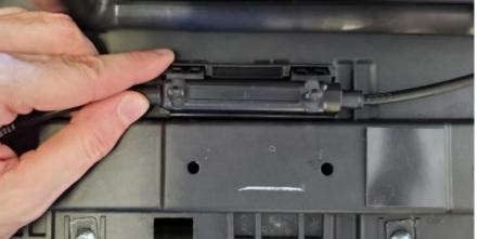
After prying off, flip the cable housing upside down as shown.
