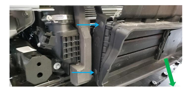
Once the Y-bracket top clips are un-done (see previous slide) you will be able to slide the entire AGS assembly downward by flexing the Y-bracket gently.
