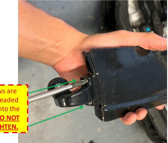
The screws are being threaded directly into the plastic. <u>DO NOT</u> <u>OVERTIGHTEN.</u>
