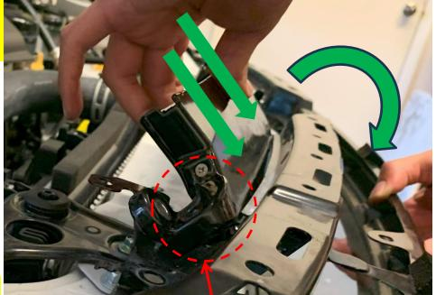
Be wary of the interference between the body and the radiator shroud at this point
