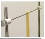
Slide the other end of the thin rod into its matching hole on the other ring stand clamp. Adjust the clamp positions so that the rod is level, allows the bouncing dart to swing freely as a pendulum and that it is at the right height to strike the middle rear of the dynamics cart at the cart's lowest point.
