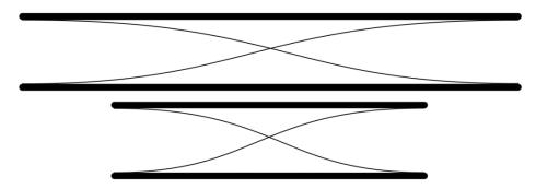
2. **Resonance:** Hum loudly over the end of a tube near and at its natural frequency. The tube will vibrate when you reach its natural frequency, in addition to amplifying the sound.
