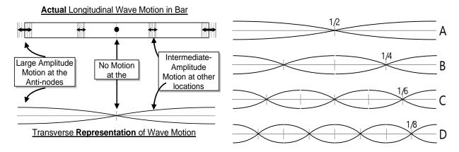
A standing wave in the rod has nodes, or regions where the rod does not vibrate at all, and antinodes, or regions where the rod is vibrating at its maximum. A rod will always have antinodes at its ends. The lower diagram shows the four standing wave patterns that will occur in the singing rods. Each pattern has antinodes at the ends of the rod and equally spaced nodes in between.
