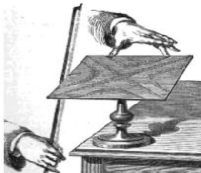
An early illustration of a Chladni Plate. Note that the thumb and fingers are used to help place the nodal lines where little movement occurs.
