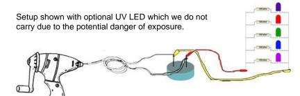
If you have the IR and UV LEDs installed: Was the Red LED really the first to come on? Better check again. You can use the viewfinder of any digital camera or cell phone to see when the IR LED lights up. What about the last LED to light? Was it the Blue?
