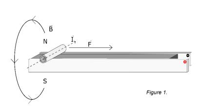
current (I), and force (**F**) for the current setup. Point your index finger along the magnetic field lines (the magnetic field is pointing *up* since the field lines travel from N to S) and extend your middle finger at a right angle to your index finger and point it along the path of the current traveling through the tube. Now stick your thumb out to find the direction of electromagnetic force. Then, send power through the circuit.
