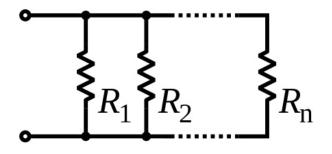
Fig. 2 Parallel circuit (of n resistors)
