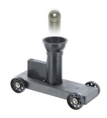
The purpose of the Ballistics Car is to show that the *horizontal component* of the ball's velocity must equal that of the car itself despite the large continuous changes in the *vertical component* of the ball's velocity. This explains how the ball can fall right back into the barrel of the launcher, given any initial speed of the car and any initial power settings of the launcher.
