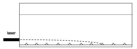
This gradual refraction results from a gradient in the index of refraction. The gradient in the index of refraction arises from the gradient in the concentration of the sugar solution.
