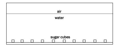
Allow 10-20 minutes for the cubes to dissolve in the undisturbed water. **Do not stir the water during this time**. The cubes will not dissolve completely, but the result will be a sugar solution concentration *gradient* from the bottom to the top of the tank. Direct the laser horizontally through the water near the top of the tank. It should be unaffected and pass through as expected.
