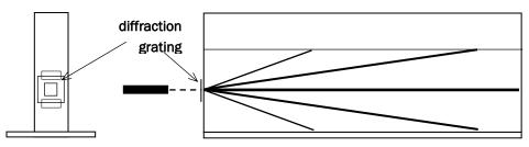
Observe the well-defined maxima as they diverge from one another in the water. By using differentcolor lasers, you can see the effect of wavelength on the diffraction pattern.
