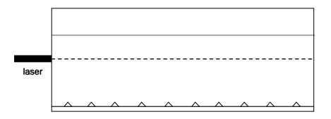
Maintain the horizontal aim as you lower the beam to deeper and deeper depths of water. As you get close to the bottom of the tank, the beam will appear to arc downward into the sugar.
