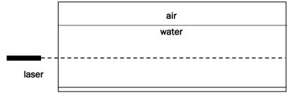
Direct the laser into the water from one end of the tank. The beam may be visible, but it will not be bright. Add a small amount of scattering agent to the tank and stir it in gently. Now shine the laser beam through the tank. Though the water still appears transparent, the beam is highly scattered and bright.
