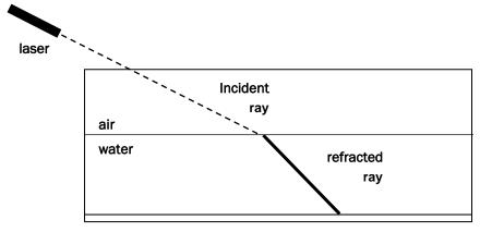
To see the difference more clearly, use the opaque, white backdrop. And use the stirring rod as a lens the spread the laser beam laterally. Aim carefully so that the laser beam can be seen on the white backdrop before and after it passes into the water.
