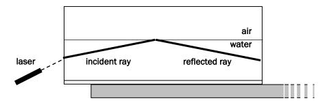
The beam will undergo total internal reflection. Vary the angle of incidence. Careful investigation will reveal the *critical angle*. If the angle of incidence from the water to the air is less than the critical angle, some fraction of the beam will emerge from the water into the air. If the angle of incidence is greater than the critical angle, total internal reflection will occur.
