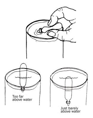
3. Use both hands to squeeze the sides of the bottle. You may have to squeeze hard depending on how you adjusted the water level inside the diver. Watch the diver sink when you squeeze the bottle, or float when you release the squeeze.
