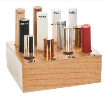
Note: The three white plastics may be difficult to identify. The translucent white plastic is nylon, the bright opaque one is teflon, and the third is PVC.
