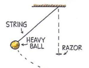
When the ball at the end of the string swings to its lowest point, the string is cut by a sharp razor.
