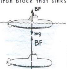
When a submarine is floating, BF equals its weight. And when it hovers while submerged at a fixed depth, BF again equals its weight—but a greater weight, due to the water added to its ballast tanks. Hence BF is greater for the submerged submarine.
