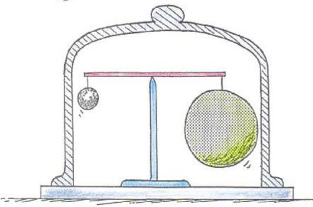
In the presence of air, the small iron ball and large plastic ball balance each other. When air is evacuated from the container, the larger ball
