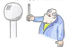
The lamp will not glow when it is held with both ends equidistant from the charged Van de Graaff generator. But when one end is closer to the dome than the other end, a current is established and it alows. Why?
