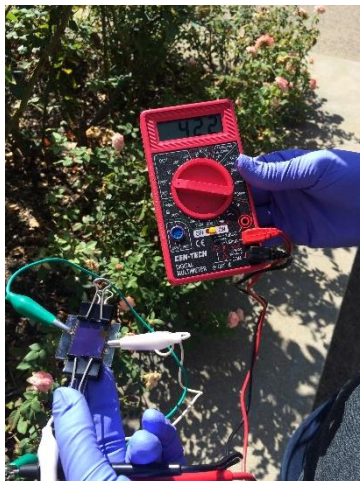
Figure 16. A completed DSSC can be tested using a multimeter.
