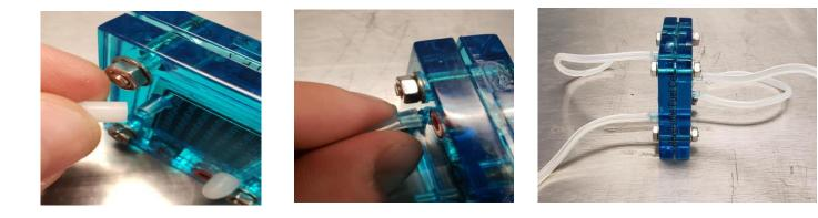
Use the syringe to add 1 mL of distilled or deionized (DI) water through the top tube next to the positive (Red) side.
