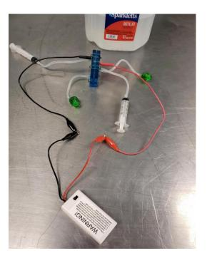
You should immediately notice small bubbles forming inside the fuel cell. After a few moments you will notice the syringes begin to fill up with what appears to be air. This is where our Hydrogen and Oxygen gasses are being stored for later use. Leave the battery on until both syringes are full. You may notice the hydrogen syringe is filling up roughly twice as fast as the oxygen syringe. The overflow valve on the hydrogen (negative) side will compensate for this offset.
