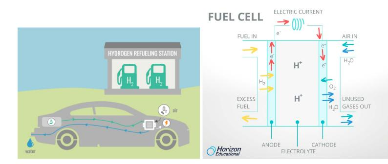
Anode: $H_2(g) \rightarrow 2H^+(aq) + 2e^-$ Cathode: $\frac{1}{2}O_2(g) + 2H^+(aq) + 2e^- \rightarrow H_2O$ Overall: $H_2(g) + \frac{1}{2}O_2(g) \rightarrow H_2O(I) + electric energy + waste heat$
