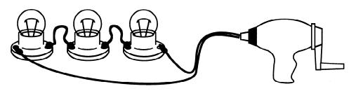
Figure 4. A hand-powered series circuit
